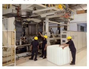
Manufacturing of rigid Intermediate Bulk Containers
