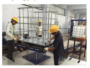
Manufacturing of cage for rigid Intermediate Bulk Containers
