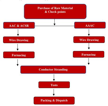
**Raw Material Purchase and Check-Points:** Aluminium alloy rod and GI core wires are the raw materials needed to make cables and conductors, and they can be acquired from a variety of authorised sources. Aluminium alloy rods are drawn to the specified needed size throughout our manufacturing process. Every step of the inspection and quality check process for purchased raw materials.
