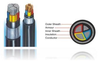
Our XLPE cables are manufactured with copper / Aluminium Conductor with XLPE Insulation, Laid up, Inner Taped/Extruded. The armouring is of galvanised mild steel wires/strips. The final outer sheath with high grade PVC. All as per relevant IS specification.
