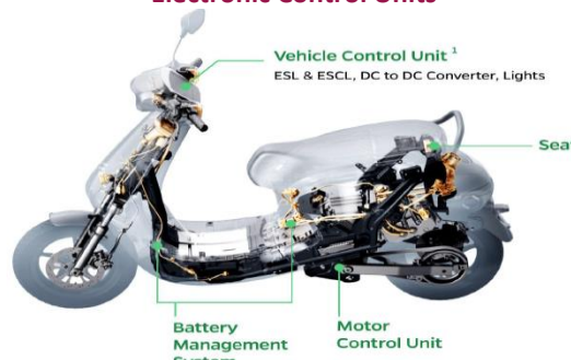
1 These control units were decentralized in Gen1
