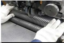
Flexible hoses are cut to the specified length as specified by the Customer's Specifications
